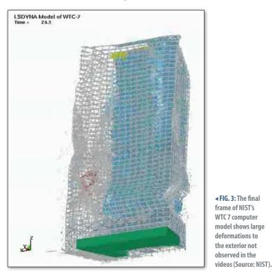
◆ FIG. 3: The final frame of NIST's WTC 7 computer model shows large deformations to the exterior not observed in the
