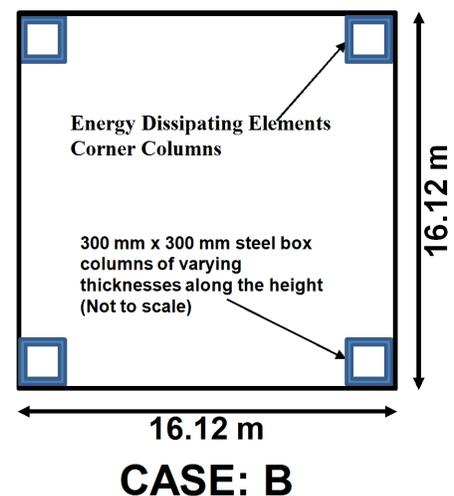
Fig. (2). Locations of Energy Dissipating Elements in Sample buildings- Case A and Case B.
