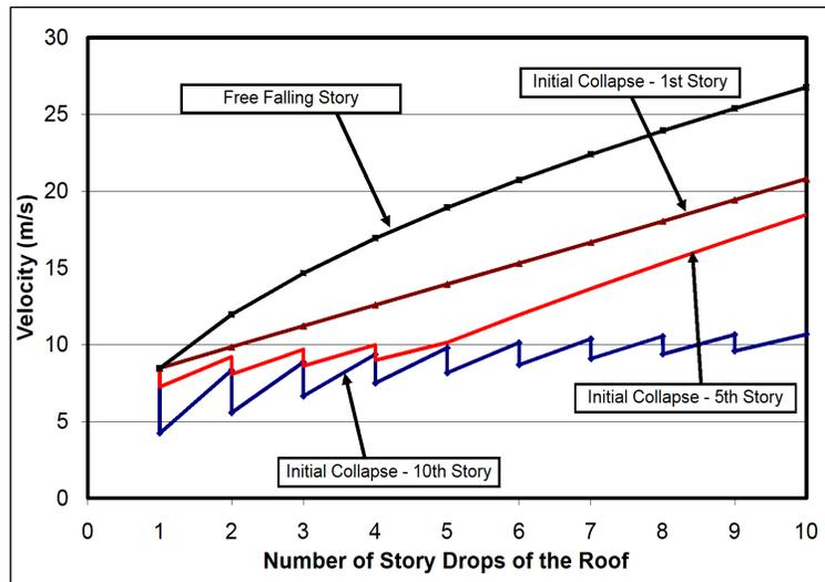
Fig. (3). Velocity with Number of Storey Drops of the Roof.
